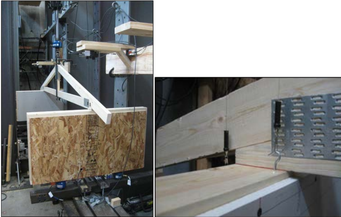
FIGURE 3. WALL CONSTRUCTION TEST SETUP
