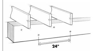
For beam depths of 18" or more, this pattern should be increased to three fasteners every 24" on center.
