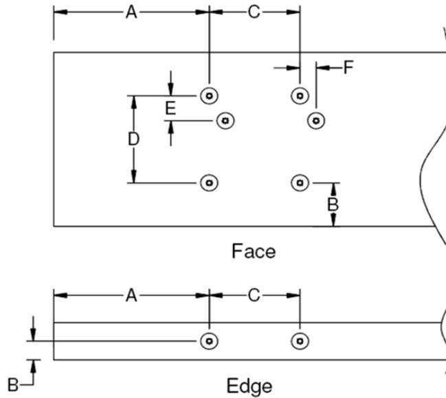
**Figure 3.** FlatLOK Edge and End Distance Requirements
