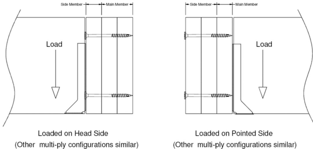
**Figure 2 .** Loading Diagram for Shear Perpendicular to Grain
