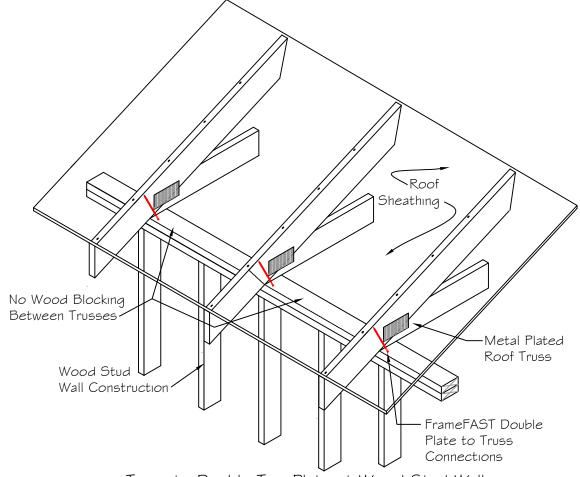
Truss to Double Top Plate at Wood Stud Wall Condition - Isometric Detail - No Wood Blocking N.T.S.
